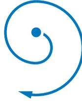
The robot will begin to explore by driving in a spiral with an ever increasing radius. When it encounters an obstacle, the robot will drive to a new location and begin to spiral again.
