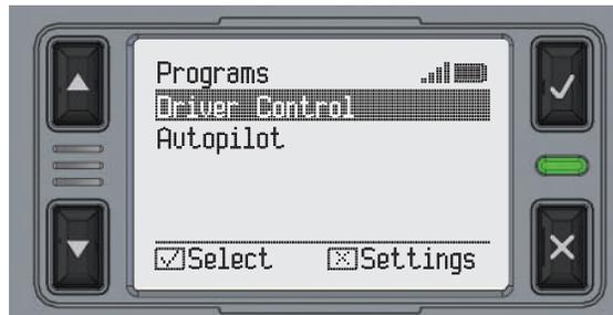
Use Up/Down arrows to highlight *Driver Control*, then press the Check button.
