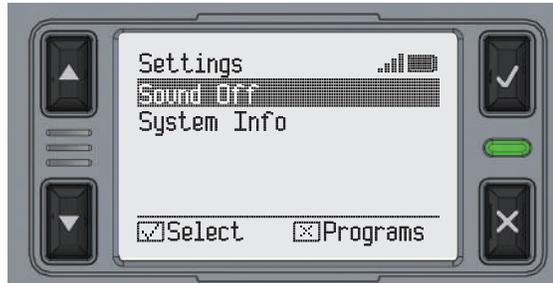
To view detailed information about the current status of the Robot Brain and the VEX Controller, use the Up/Down arrows to highlight the **System Info** row and press the Check button.
