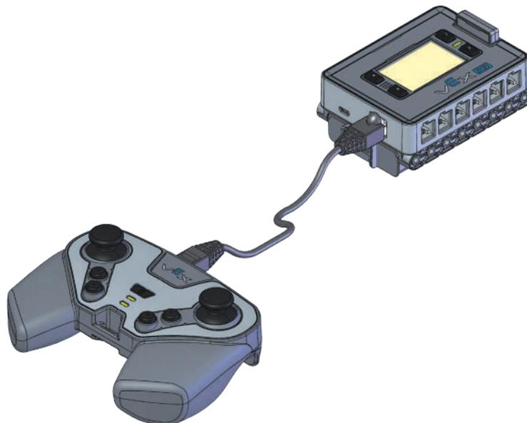
Turn the Robot Brain ON by pressing the Check button. The Controller will automatically link and pair to the Robot Brain. The Tether Icon will appear on the Robot Brain LCD screen.
