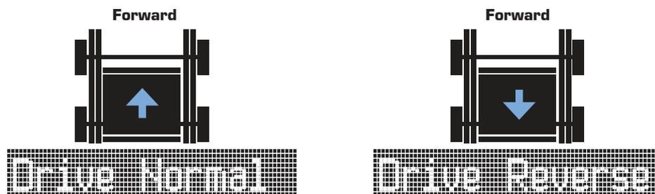
Sometimes, you may want to change which side of a robot is considered the front to make it easier to drive. The *Drive* option allows you to control this, so that pushing upwards on a joystick axis always makes your robot drive forward. To change this setting, highlight the *Drive* row, and press the Check button to cycle between *Normal* and *Reverse*.
