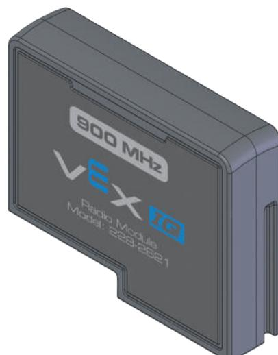
**Ensure there is no battery plugged into the Robot Brain.** Slide the Radio into the Radio Socket. Orient the Radio so its VEX logo is away from the LCD screen. Press it in firmly.
