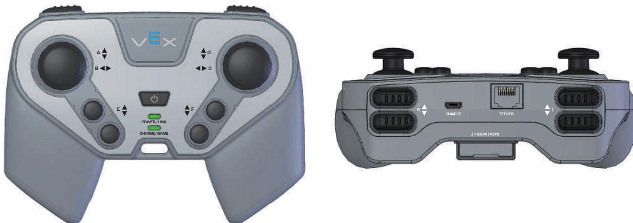
The Controller also has 4 pairs of buttons labeled E, F, R and L. These buttons turn the motors on at full speed in one direction. Each button pair controls the clockwise and counterclockwise direction of the motor.
