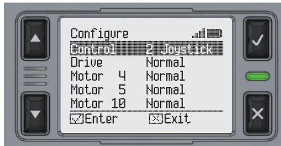
Use Up/Down arrows to highlight *Configure*, then press the Check button.
