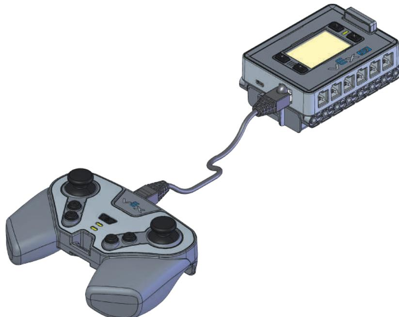
Controller Battery charging will take about 4 hours. While the Controller Battery is charging, the Charge/Game LED on the Controller will be solid red. When the Controller Battery is fully charged, the LED will change to solid green. See [page 95](#) for detailed LED color diagram.
